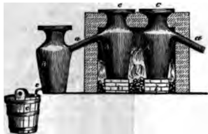
Distillation of Native Sulphur.
